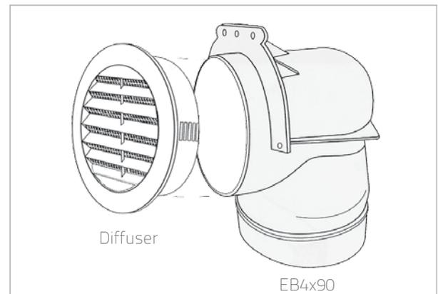
Installation using Primex's 'Squeeze Elbow'
